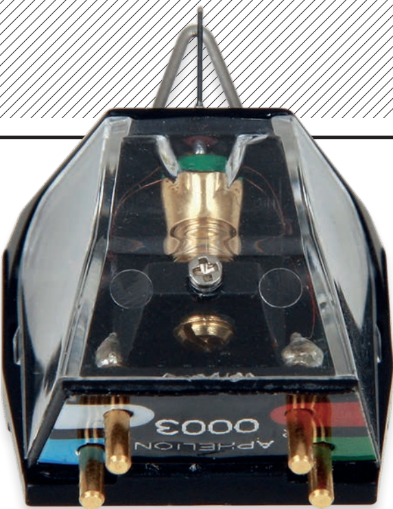
LEFT: Another view of Rega's long boron cantilever and substantial neodymium/iron magnet yoke. The cartridge pins are gold-plated and well spaced to accommodate most tonearm leads/tags
